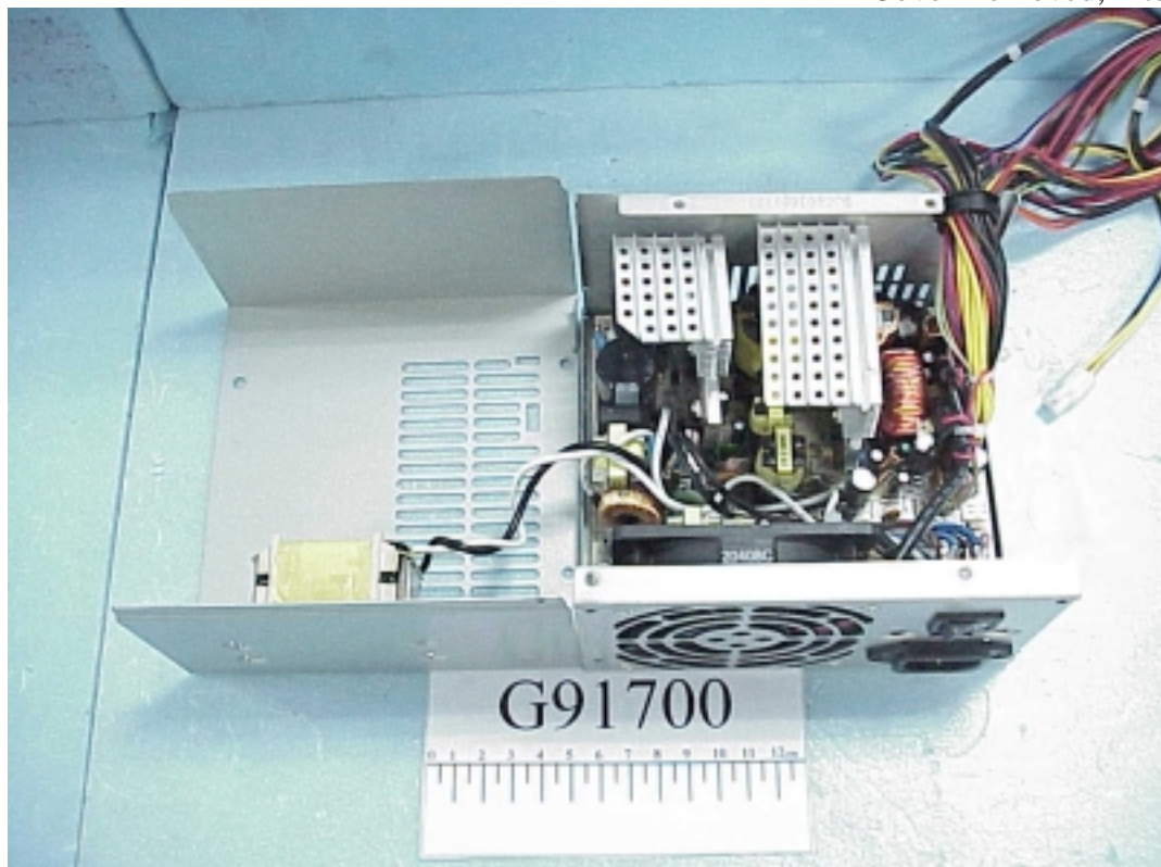
Figure 4 M/N : ATX-250GT Cover Removed, Internal View
